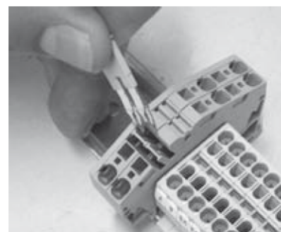
Removal of shunt to deactivate a heater (reduction of 300 W)
